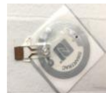
Elvikon sensor platform: A simple configuration of the label with counterparts IDE - NFC tag and its reality.
